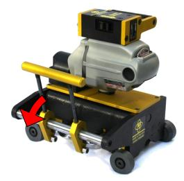
It is important to remember to use extreme caution when reaching the edge of the roof. Stop and disengage the locking handle of the seamer while the wheels remain on the roof panel. Do not run the seamer within 6" of the end of a panel, beyond the end of a panel or over a previously seamed area. Use your hand crimpers to finish any area that the seamer may not be able to complete, such as against a ridge cap, end cap or at a pitch change in the roof.
